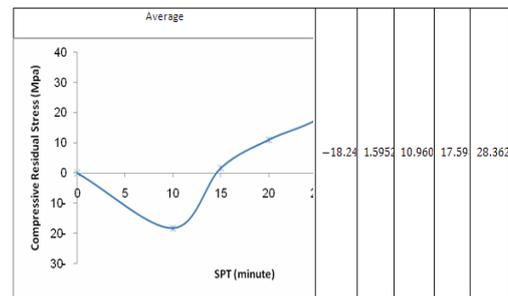
**Fig. (7): Effect of shot peening time on compressive residual stress**
