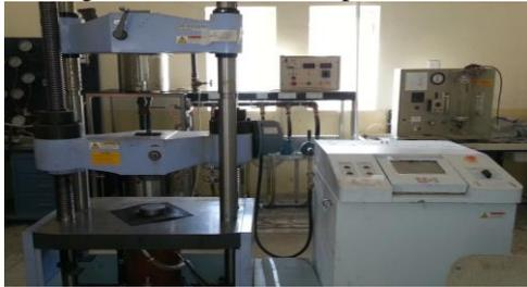
**Fig. (2): Tensile test machine type (SHIMADZU-600KNI)**
