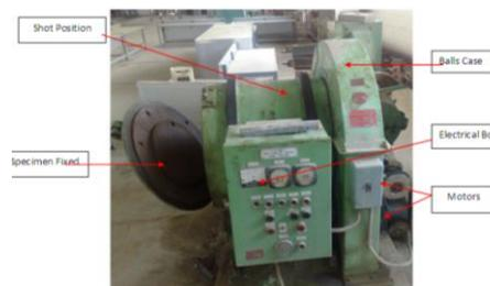
Fig. (1): Shot peening device
