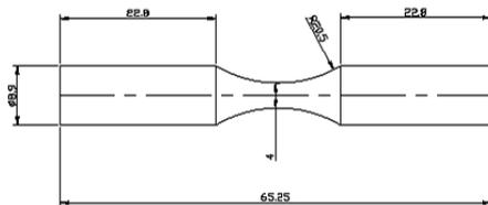
**Fig. (4): Rotating bending fatigue testing specimens**
