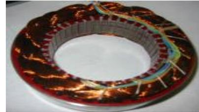
**Figure 6: Stator of PMSM**
