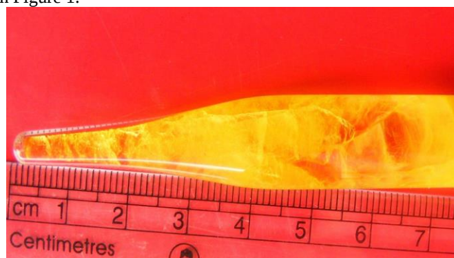
Figure 1. Photograph of the LVP uniaxial single crystal
