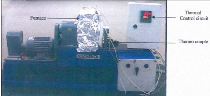
Fig. (2) b. the fatigue-creep testing machine with furnace
