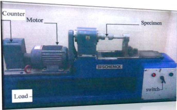
Fig. (2) a. the fatigue-creep testing machine
