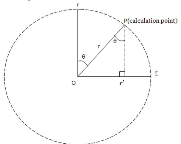
**Fig 2. Calculation of radial distances from the centre of the source**
