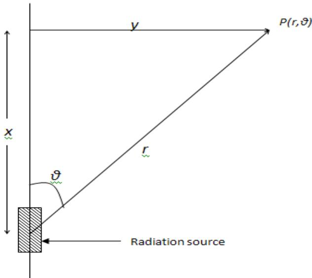
**Fig.1. Schematic representation of an HDR brachytherapy source showing the geometric definition of r and theta for a filtered radiation source**
