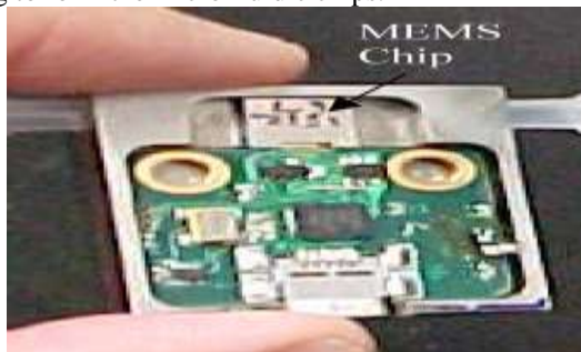
Fig 2. Uncapped microtube resonator chip (4)
