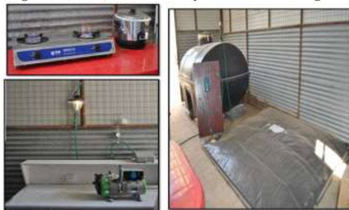
Figure 7. Pilot-scale biogas production from portable solar anaerobic digestion
