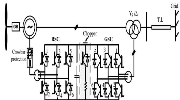
Fig 1. Typical configuration of DFIG System under Study
