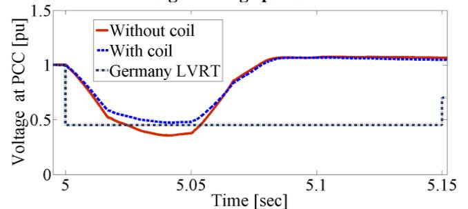
**Fig. 5 PCC voltage compliance with Germany grid codes**
