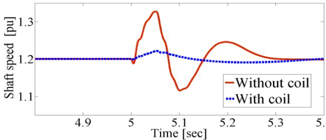
Fig. 8 DFIG shaft speed
