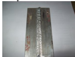
Figure 11. friction stir welded aluminum alloy H20 straight cylindrical tool.
