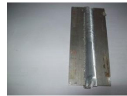
Figure 9 .friction stir welded aluminum alloy H20 triangular tool
