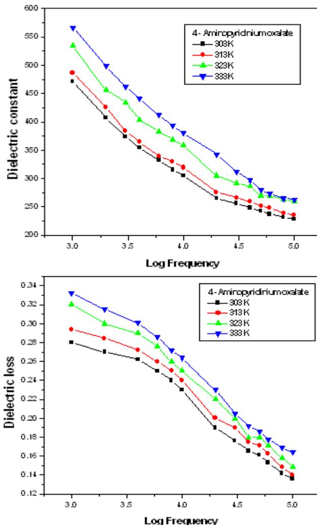
Fig.9. Variation of (a) dielectric constant and (b) dielectric loss with temperature and frequencies for 4APO crystal.
