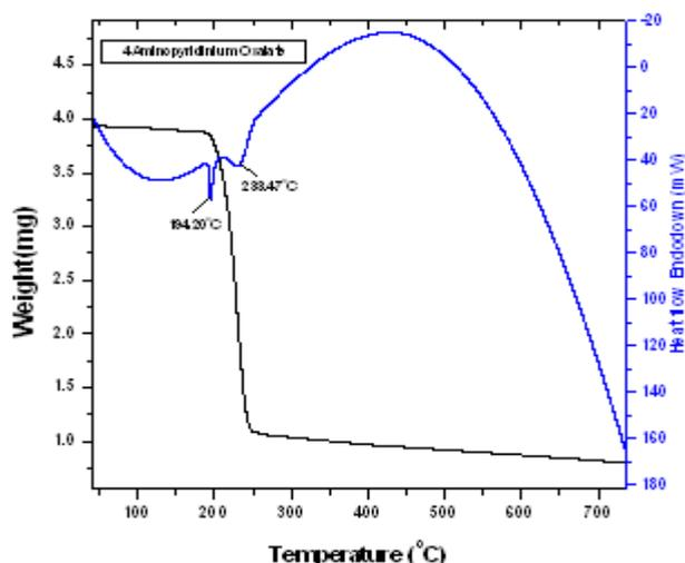
Fig.6. TGA/DTA curve of 4APO crystal
