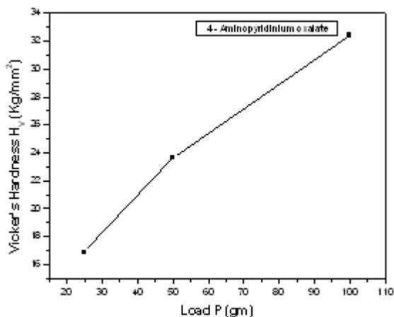
Fig.7. Load ( $P$ ) vs. hardness number ( $H_V$ ) of 4APO crystal
