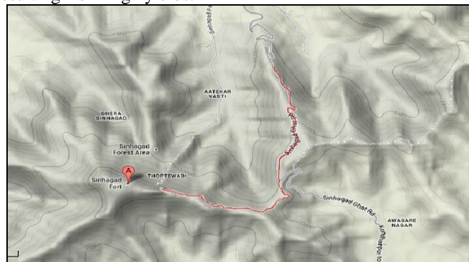
Figure 5. Contour map of the region; Red line showing the stretch of 3.6 KM which is contributing water for Aatekar Vasti
