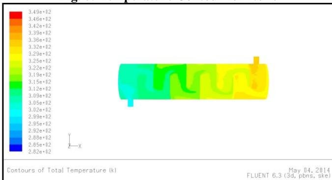
Fig. 9: Temperature Contour for Nb=8
