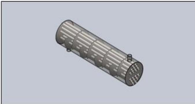
**Fig. 4: Equally spaced 8 baffles**
