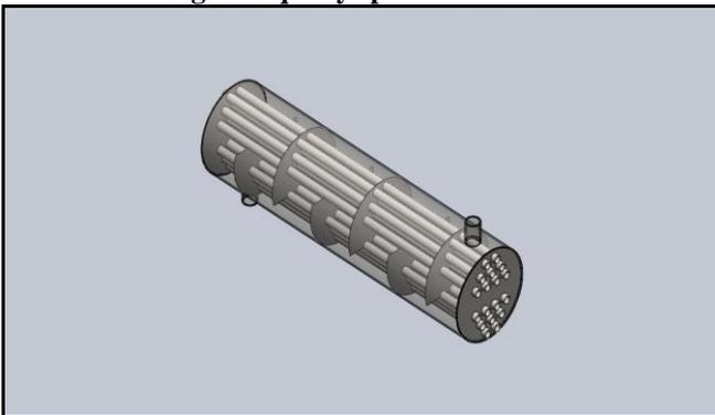
**Fig. 3: Equally spaced 6 baffles**
