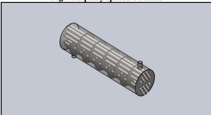
**Fig. 5: Equally spaced 10 baffles**
