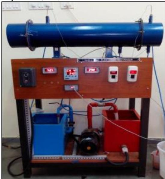
**Fig. 1: An unit of STHE in VTU Gulbarga**
