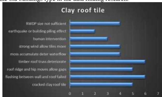
Figure 2. Identified factors leading to water seepage on clay roof tile for the case studies
