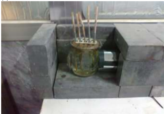
Fig. 1: Experimental arrangement for void fraction measuring equipment
