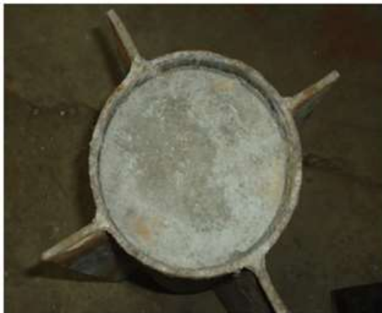
Fig 5. Typical bond failure of CFT
