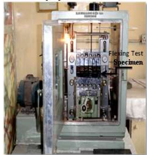
Fig.(2): De Mattia Flexing Machine Test
