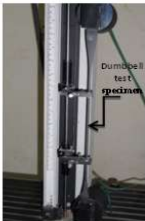
Fig.(1): Monsanto T10 Tensometer.
