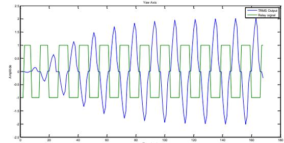
**Figure 5: Response of relay feedback test simulation for yaw axis**
