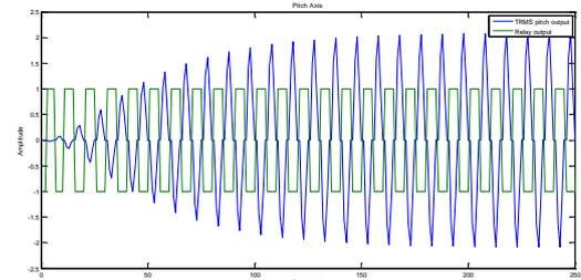
**Figure 4: Response of relay feedback test simulation for pitch axis**
