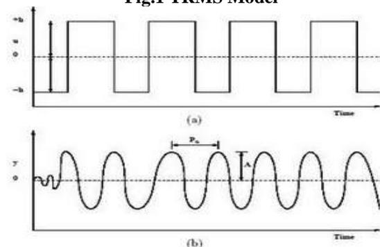
Fig.2 Waveforms of relay output in closed loop
