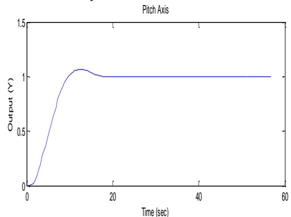
**Figure 6: Simulation closed-loop response with PID controller tuned using Ziegler Nicholas tuning rule for pitch axis**
