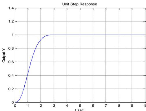
**Figure 10: Simulation of closed-loop response with State feedback Integral controller for yaw axis.**
