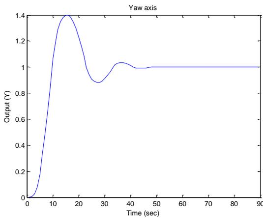
**Figure 7: Simulation closed-loop response with PID controller tuned using Ziegler Nicholas tuning rule for yaw axis**
