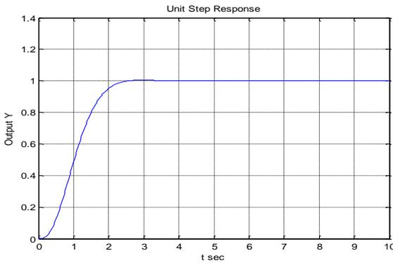
**Figure 9: Simulation of closed-loop response with State feedback Integral controller for pitch axis.**
