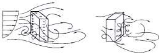
Fig 2.2 A typical bluff building
