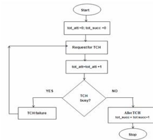
Figure 3. Flow chart of fixed channel Allocation Algorithm
