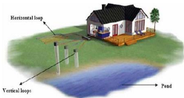
Figure 1. Using the soil, bedrock or groundwater as the heat source
