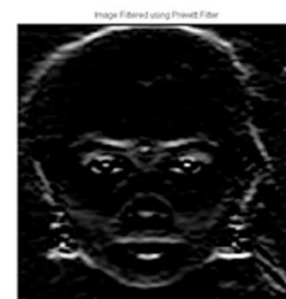
Figure 7. Image shown in Figure 6 Filtered using Prewitt filtering technique
