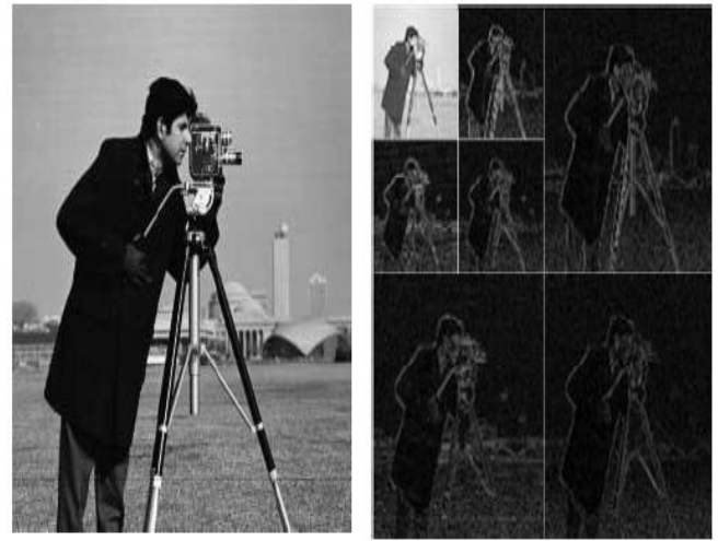
Figure 3. Illustration of 2 level DWT for an image
