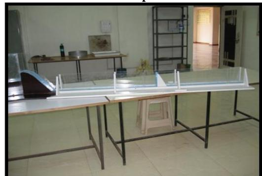
Fig 5. View of main weir, apron, stepped weir and Tail channel
