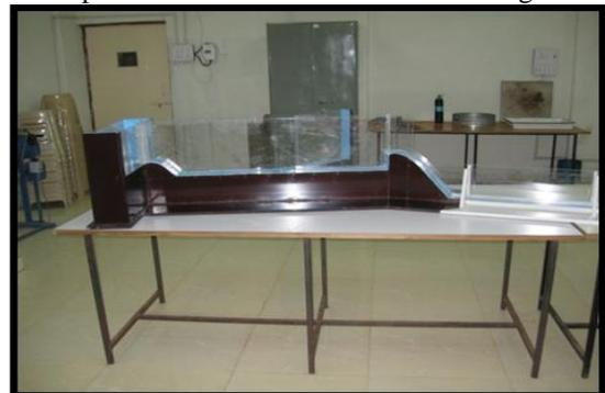
Fig 4. View of model with escape structure and Main Weir
