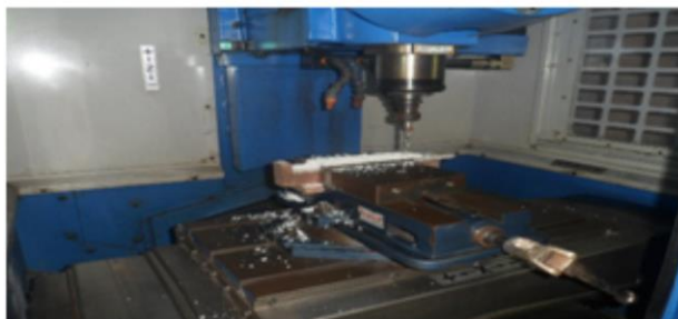
Figure 4. GFRP composite drilling operation on VMC
