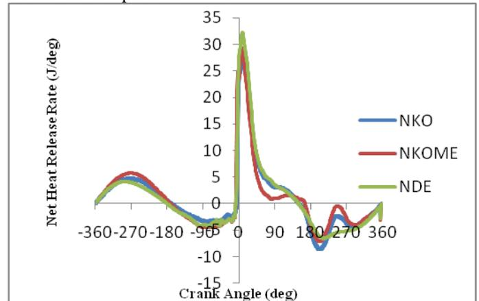
Figure 8. Variation of heat release rate with crank angle.
