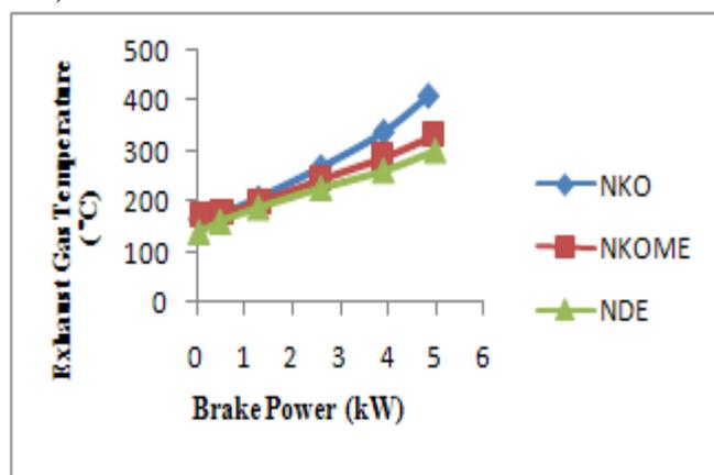
**Figure 3. Variation of EGT with brake power.**
