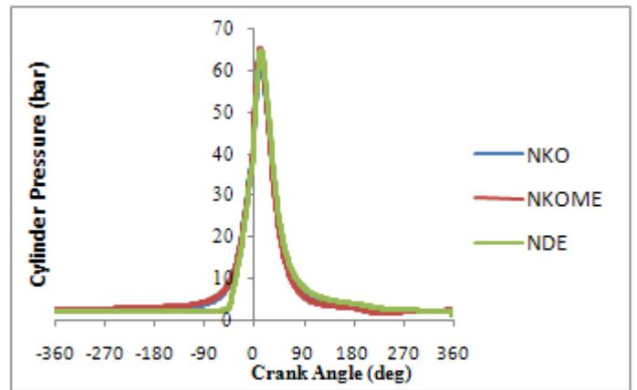
Figure 7. Variation of cylinder pressure with crank angle.
