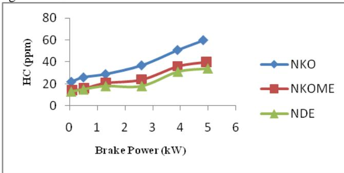
Figure 5. Variation of Hydrocarbon with brake power.
