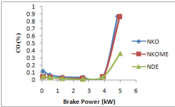
Figure 4. Variation of CO with brake power
