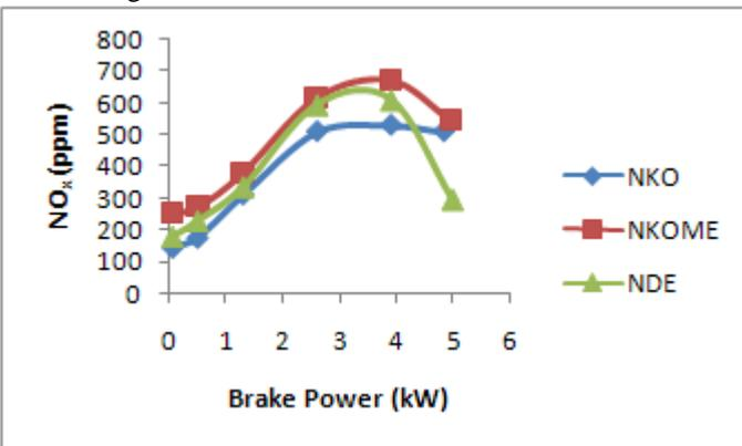
Figure 6. Variation of NOx with brake power.
