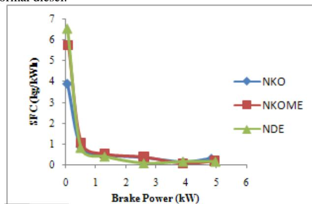
**Figure 2. Variation of SFC with brake power.**
