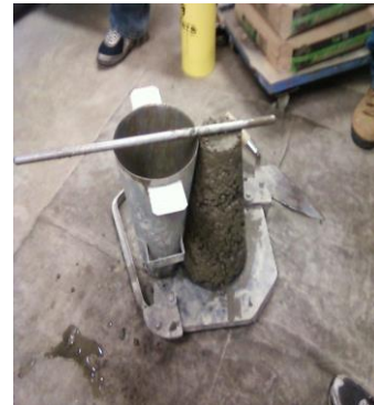
Fig 4(b). Placement of concrete with transit mixers of slump of 25 mm
