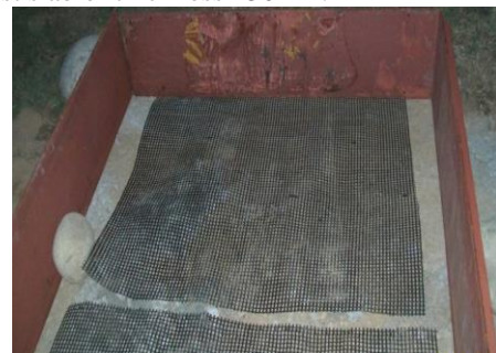
Fig 5(a). Glass grid at 100mm from bottom.
