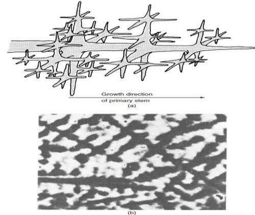
**Figure 2. Dendritic growth. (a) Classical concept of a dendrite, (b) dendritic microstructure in carbon-chromium steel. X5 approx [55]**
