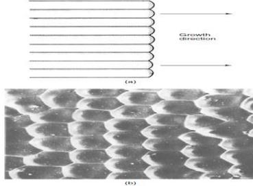
**Figure 3. Cellular substructure formed by undercooling. (a) Structure in growth direction, (b) hexagonal cells on growth interface [55]**
