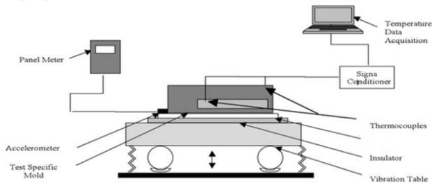
**Figure 1. Schematic illustration of the assembled apparatus for applying mechanical vibrations to a permanent steel mold. [ 89]**
