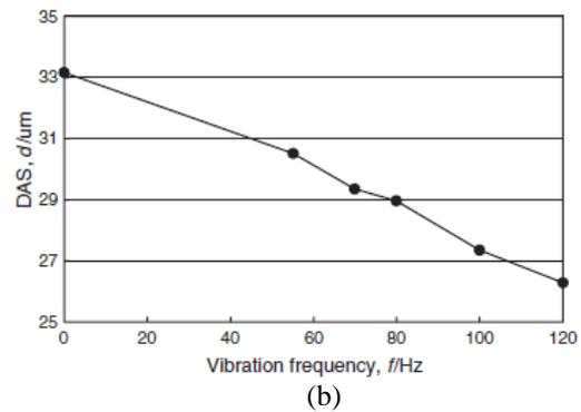
Figure 5. (a)Effect of vibration frequency on the cooling rate of the melt at bottom area. (b)DAS (Dendrite Arm Spacing) in the outer region of specimen as a function of the vibration frequency [86]
