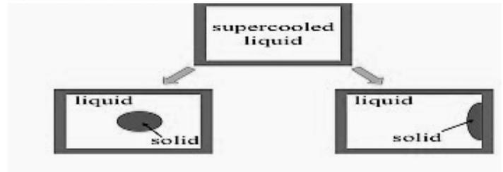
**Figure 4. Homogeneous nucleation and Heterogeneous nucleation [58]**
