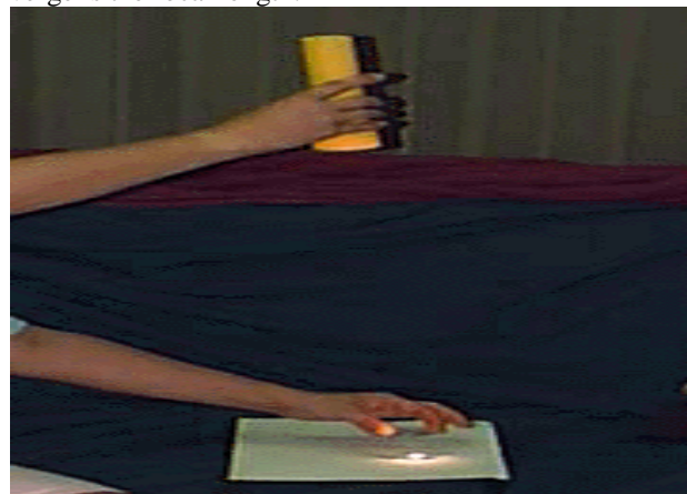
Fig. 3.2. Determining the focal length of the objective lens
