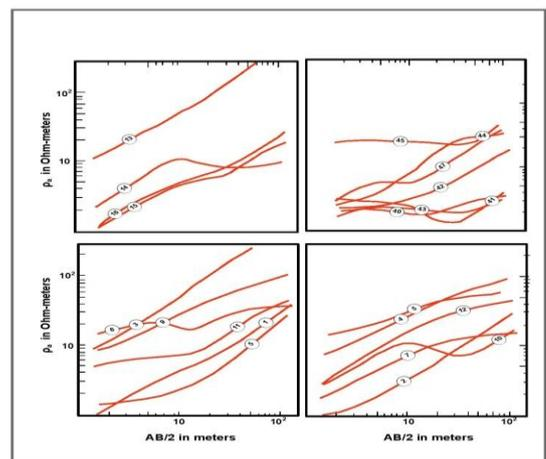
**Fig. 4. Field curves of Vertical Electrical soundings**
