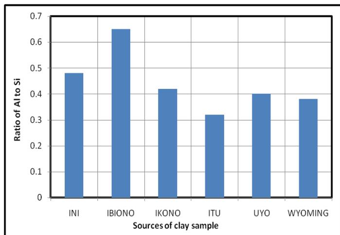
**Figure 3: Comparison of the Al to Si ratio for the clay samples and Wyoming Bentonite**
