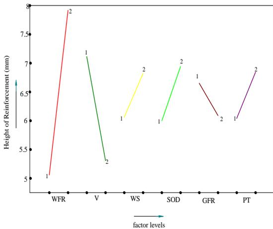
Figure 6 Main effects of parameters on Height of reinforcement (R)
