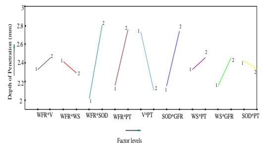
Fig 11 Effect of 2-factor interactions on depth of penetration (P)
