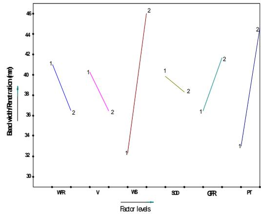
Fig 8. Main effects of parameters on weld penetration shape factor (W/P)
