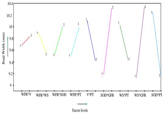
Fig. 13 Effect of 2-factor Interactions on bead width (W)
