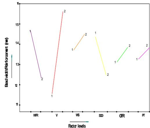
Fig 9. Main effects of parameters on weld reinforcement form factor (W/R)
