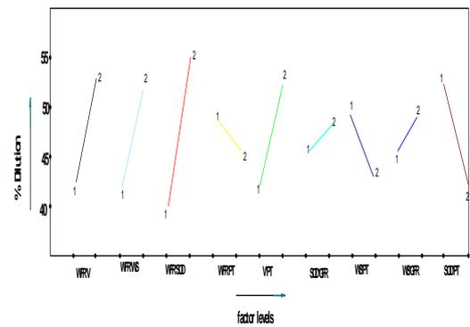
Fig. 16 Effect of 2-factor interactions On weld reinforcement form factor (W/R)
