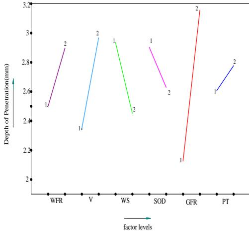
Fig 5. Main effect of factors on depth of penetration (P)
