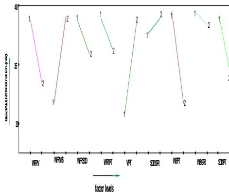
Fig. 14 Effect of 2-factor interactions on weld penetration shape factor (W/P)
