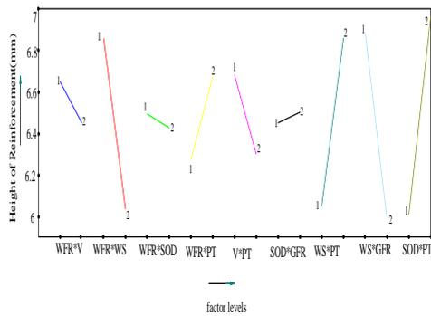
Fig. 12 Effect of 2-factor interactions on height of reinforcement (R)
