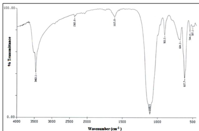
**Fig 4b. FTIR of Cd-Monoethanolamine at 500°C**
