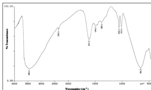
Fig 2a. FTIR of Ni-Monoethanolamine at  $150^\circ\text{C}$
