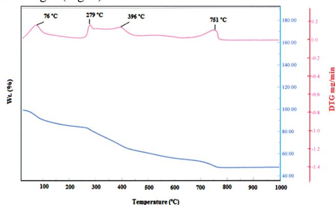
Fig 2. TG/DTG of Ni-monoethanolamine
