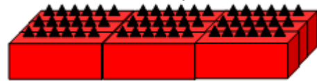
Figure 2. Shows the main prototype design of piezoelectric flooring where the single panel is combined into a set of 9 panels consisting of 54 Piezo crystals as single unit
