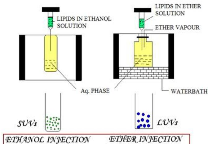
Fig 13. Method of preparation of liposomes by solvent dispersion
