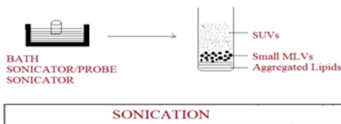
Fig 10. Method of preparation of liposomes by sonication
