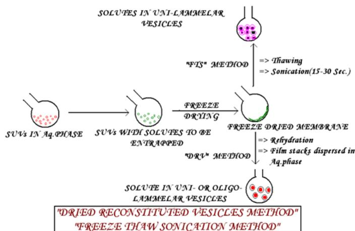
Fig 12. Method of preparation of liposomes by freeze thaw sonication
