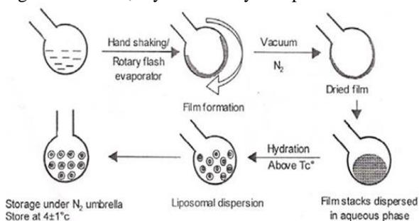
Fig 9. Method of preparation of liposomes by Hand shaking method
