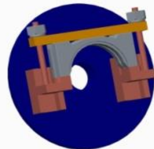
Figure 2.2. 3D view of rotary fixture with Clamped work-piece
