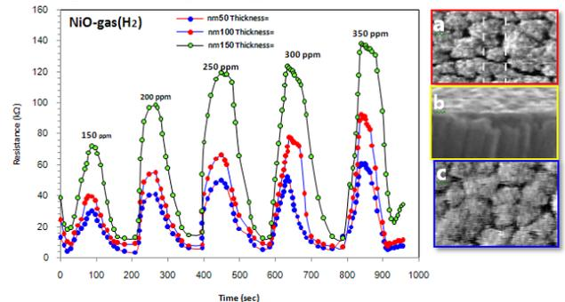
**Fig 3a.resistance of NiO thin films deposited by RF-reactive sputtering varying with time and for different thickness and at operating temperature (150C°). (a)50 nm thickness top view (b)100 nm thickness cross section view(c)150 nm top view of SEM (surface electron morphology)**
