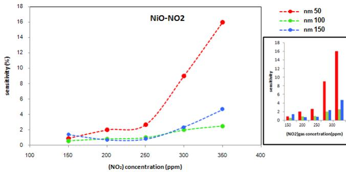
**Fig 4a.** Sensitivity of NiO thin films with different NO<sub>2</sub> gas concentration and thickness variation as deposited by RF-reactive sputtering and at operating temperature (150C°)
