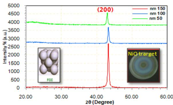
**Fig 1. X-Ray diffraction pattern of NiO thin films deposited by RF-reactive sputtering**
