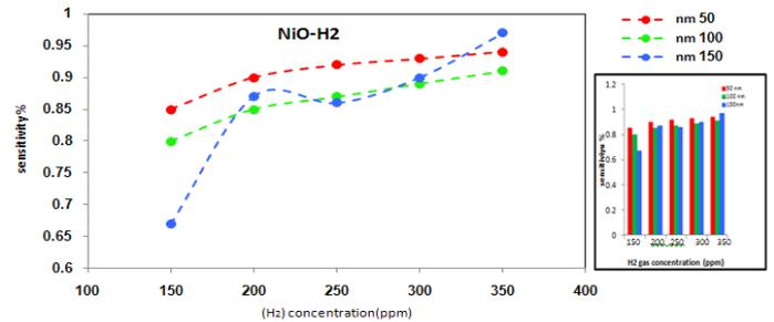
**Fig 4b.** Sensitivity of NiO thin films with different H<sub>2</sub> gas concentration and thickness variation as deposited by RF-reactive sputtering and at operating temperature (150C°).
