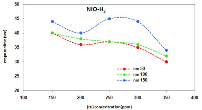
**Fig 5b.** Response time of NiO films deposited by RF-reactive sputtering to H<sub>2</sub> gas with deferent concentration and at operating temperature (150 C°)
