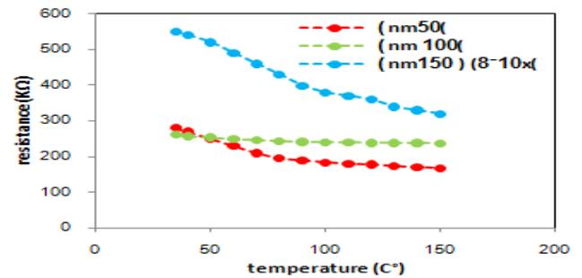
**Fig 2. Electrical resistance of NiO thin films as function of temperature as deposited by RF-reactive sputtering Sensing properties**
