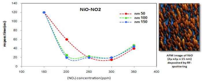
**Fig 5a.** Response time of NiO films deposited by RF-reactive sputtering to NO<sub>2</sub> gas with deferent concentration and at operating temperature (150 C°)
