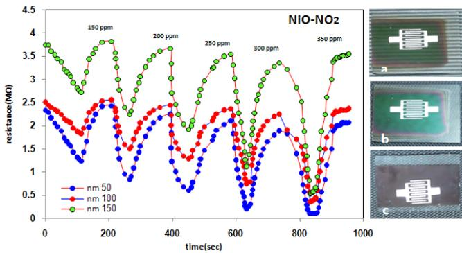
**Fig 3b and Fig 3a** resistance of NiO thin films deposited by RF-reactive sputtering varying with time and for different thickness and at operating temperature (150C°)(a)50 nm(b)100 nm (c)150 nm
