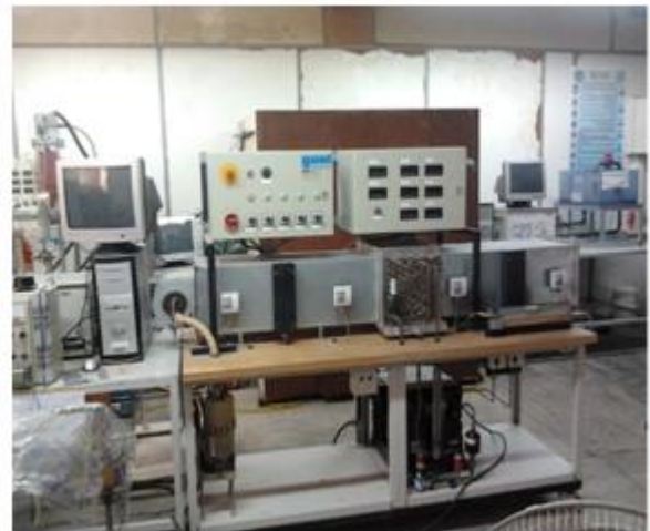
Fig 2. Air-conditioning system, ET600
