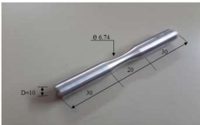
**Fig 1. Dimension of fatigue test specimen according to DIN 50113.(All dimension in mm)**
