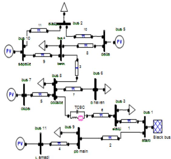
Fig 6. Simulation of 11bus, 330kv South East Nigerian network with TCSC inserted optimally
