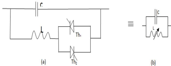
**Fig 1. TCSC configuration (a) Basic circuit (b) The equivalent circuit**
