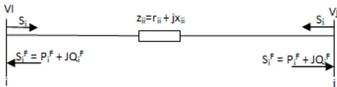
Figure 4. Static power injection model of TCSC
