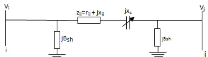
**Figure 3. Static model of line with TCSC**
