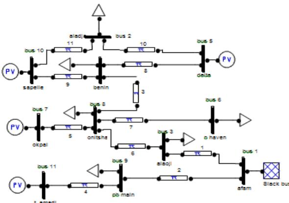
Fig 5. Base case simulation of 11bus, 330kv South East Nigerian network (without any insertion
