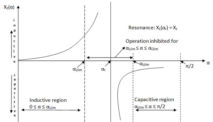
**Figure 2. The Impedance vs. Delay angle  $\alpha$  characteristic of the TCSC**
