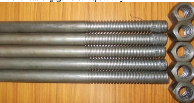
Fig 5. Threaded rod of a modified square thread after the testing
