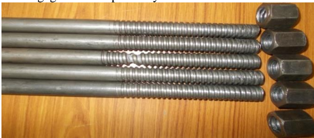
Fig 4. Threaded rod of a ACME thread after the testing
