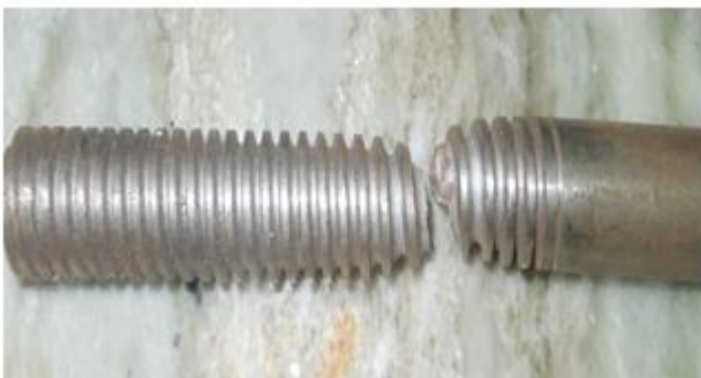
Fig 6. Failed mild steel IS2062 tie rod with six engaged threaded turns
