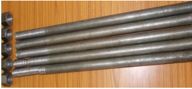
Fig 3. Threaded rod of a buttress thread after the testing
