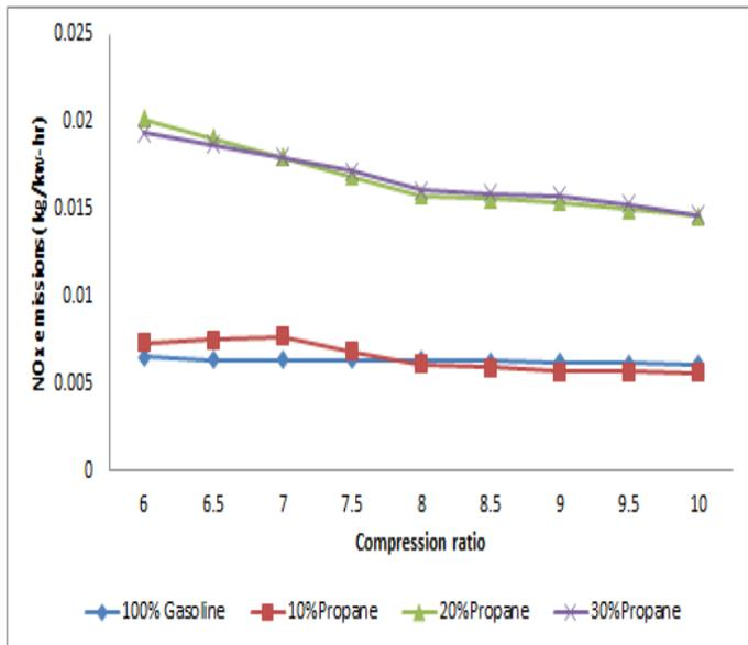
**Fig 4. Shows the graph between NOx and Compression ratio**
