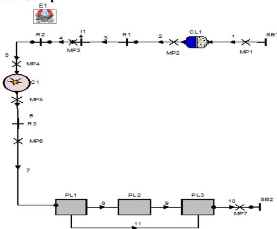
**Fig A. Layout of Gasoline engine model**
