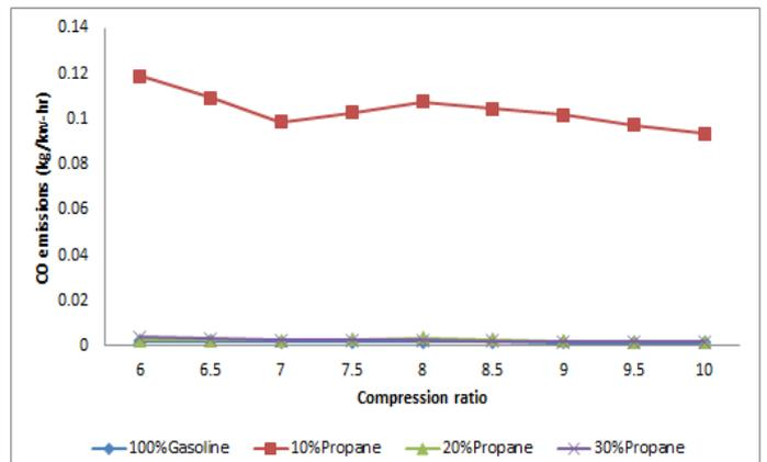
**Fig 5. Shows the graph between CO emissions and Compression ratio**
