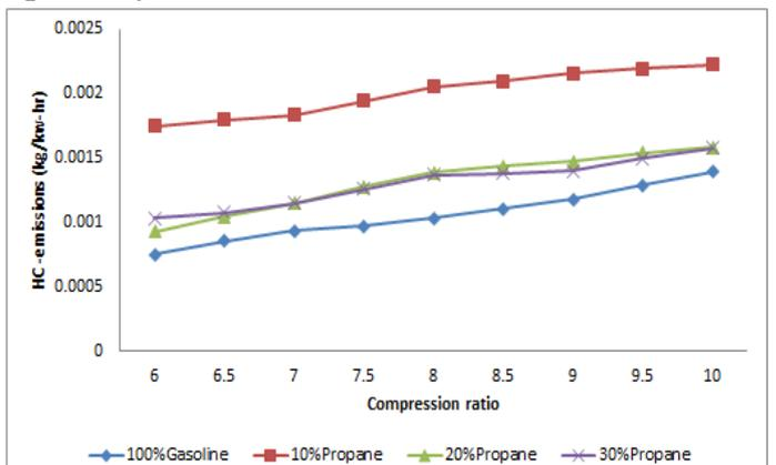
**Fig 6. Shows the graph between HC emissions and Compression ratio**
