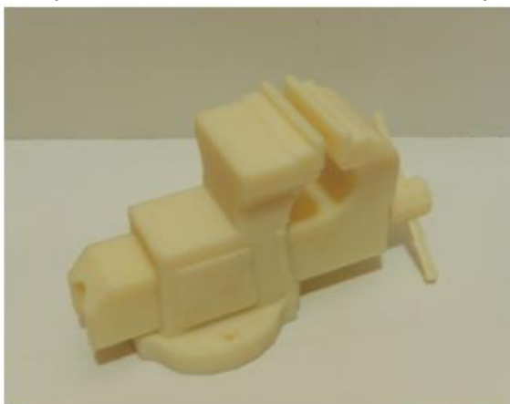
Fig 7.7 Assembly of movable jaw and modified fixed jaw
