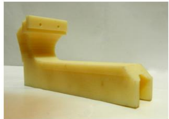
Fig 7.4 Movable jaw manufactured on RPT machine
