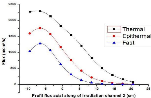
Figure 6. Axial Profile Flux distribution of channel 2
