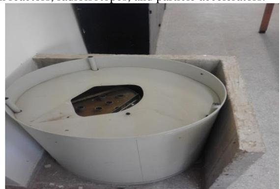
Figure 1. picture of Source Ra-Be in USMBA-FSDM-Fez Morocco of Ra-Be neutron source assembly
