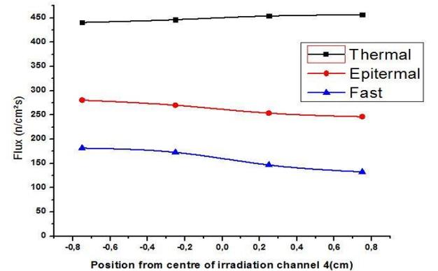
Figure 14. Radial Profile Flux distribution of channel 4
