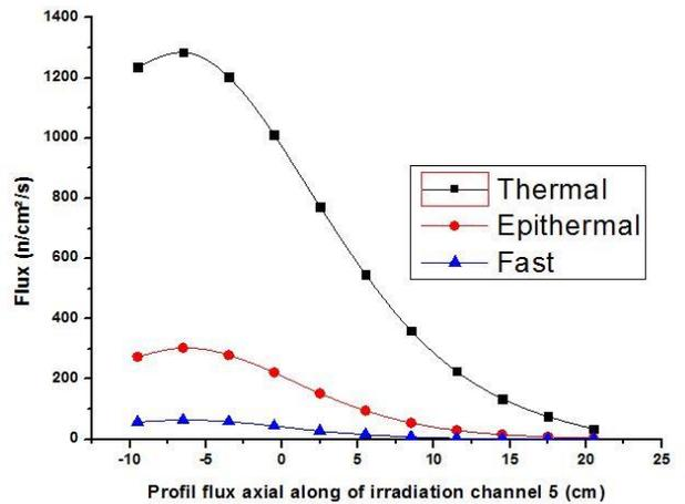
Figure 9. Axial Profile Flux distribution of channel 5
