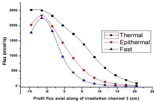
Figure 7. Axial Profile Flux distribution of channel 3
