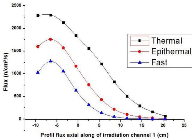
Figure 5. Axial Profile Flux distribution of channel 1
