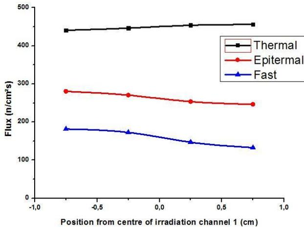
Figure 11. Radial Profile Flux distribution of channel 1
