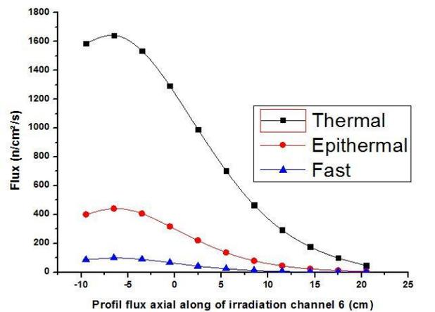
Figure 10. Axial Profile Flux distribution of channel 6
