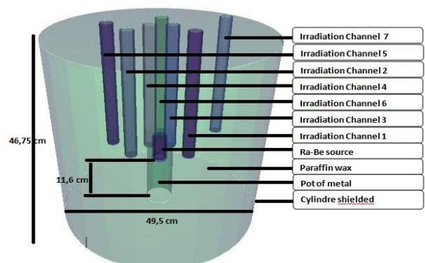
Figure 2. Schematic of Ra-Be neutron source assembly
