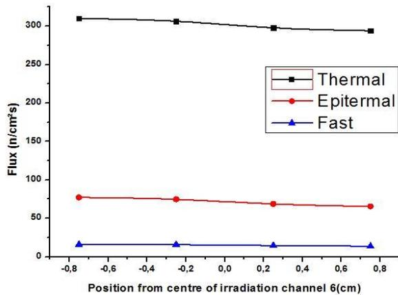
Figure 16. Radial Profile Flux distribution of channel 6
