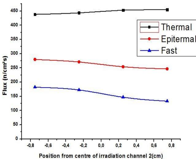
Figure 12. Radial Profile Flux distribution of channel 2
