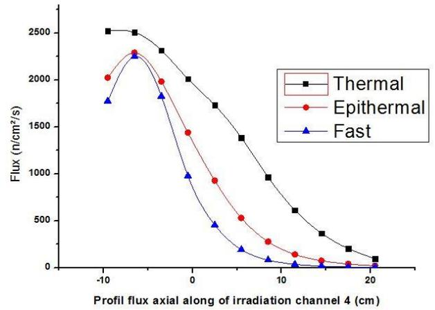
Figure 8. Axial Profile Flux distribution of channel 4
