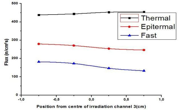
Figure 13. Radial Profile Flux distribution of channel 3
