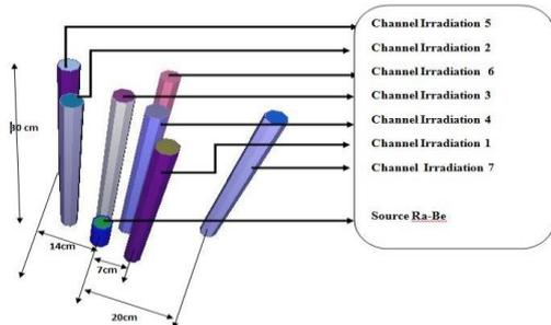
**Figure 3. Schematic of Ra-Be neutron source assembly**
