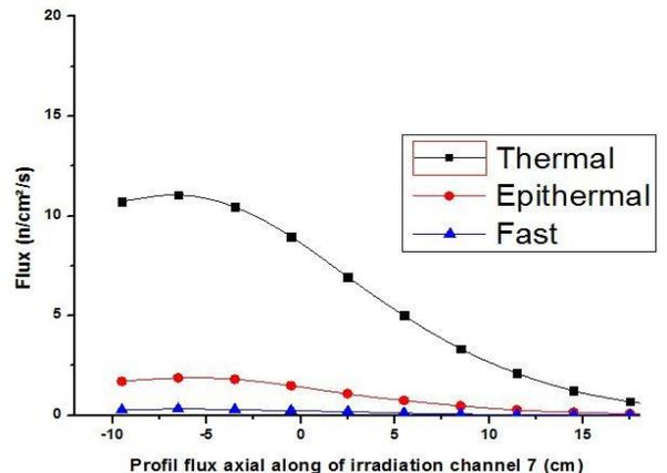
Figure 11. Axial Profile Flux distribution of channel 7
