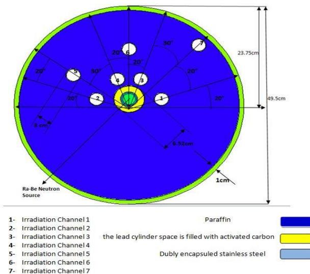
**Figure 4. Schematic cross-sectional view of the <sup>226</sup>Ra-Be neutron source assembly**
