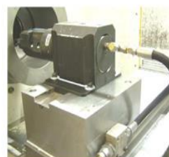
Fig 8. Setup for high pressure coolant delivery to the tool tip [2]
