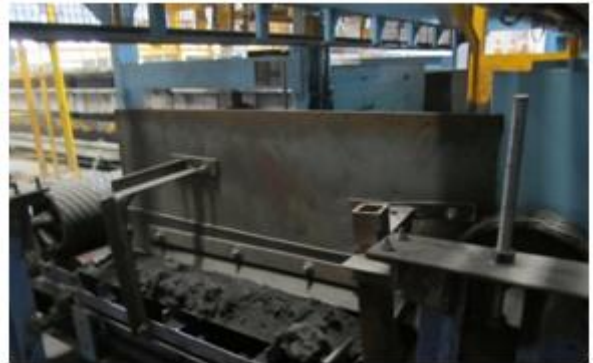
Photograph 3.5. Skirt plate to prevent sand wastage
