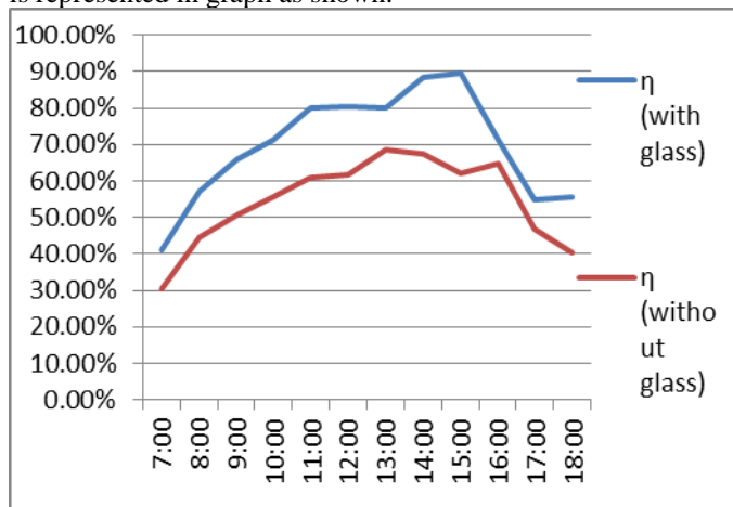
Figure 6. Graph represent the variation in efficiency of the parabolic trough.
