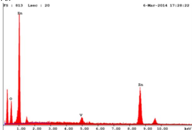
**Figure 3. EDS of sample V-doped ZnO**
