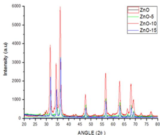
**Figure 1. XRD patterns of pure and V-doped ZnO samples.**
