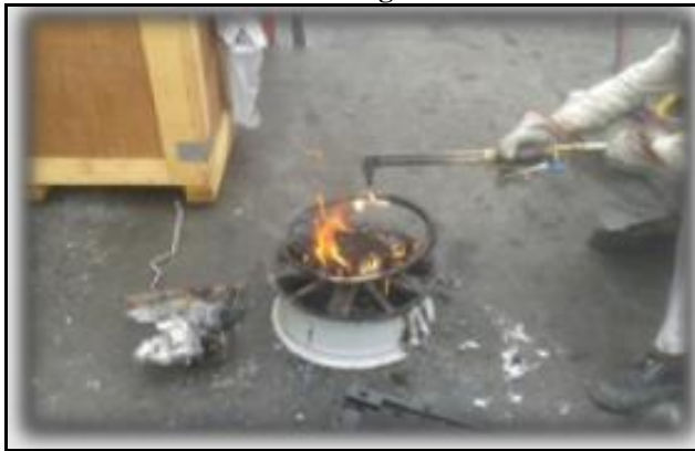
Figure 2. Shows the removal of coating material
