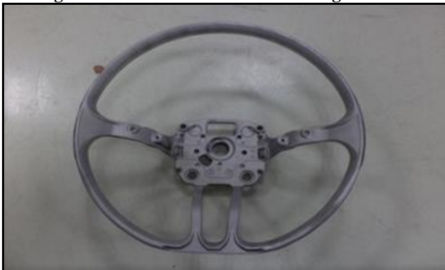
Figure 3. Depicts the aluminum ring without coating material
