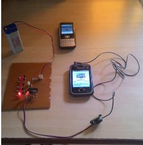
Figure 9. A GSM modem connected to DTMF card.
