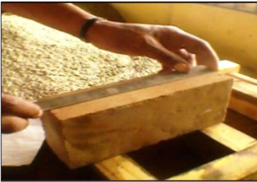
Plate 19. Measuring the Reduction in Size of the Brick Specimen after 21 Days of Air Drying
