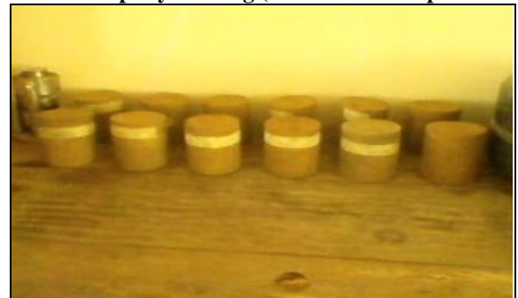
Plate 13. Cubed Test Specimens Prepared for Mechanical Property Testing (unconfined compressive test).
