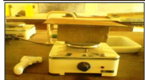
Plate 11. Thermometer, hot plate, brick specimen and cold plate
