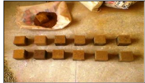
Plate 13. Cubed Test Specimens Prepared for Mechanical Property Testing (unconfined compressive test).
