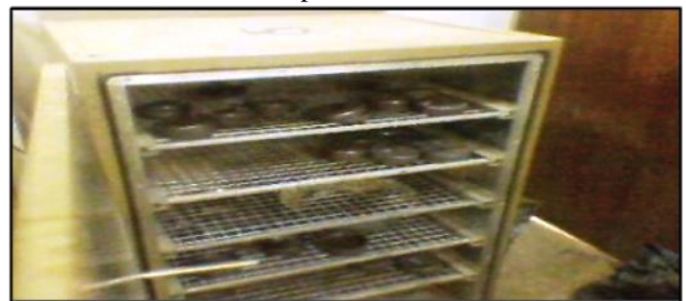
Plate 17. Containers with Samples in the Oven Set at 110°C for 24 Hours Drying
