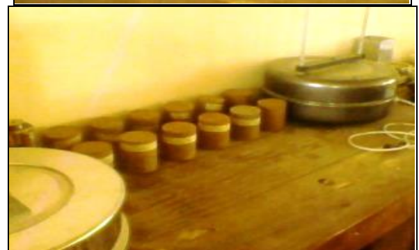
Plate 14. Cylindrical Test Specimens Prepared from Compaction Test for Physical Property Testing
