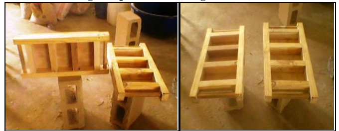
Plate 9. Detachable wooden brick mould of size 215 x 102.5 x 65mm
