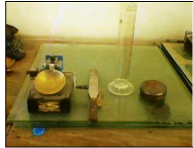
Plate 8. Limit device, spatula, grooving tool, cylinder, lid and glass plate (Atterberg Limits)
